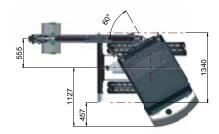
Fig. 3: Transport position - trailer transport
