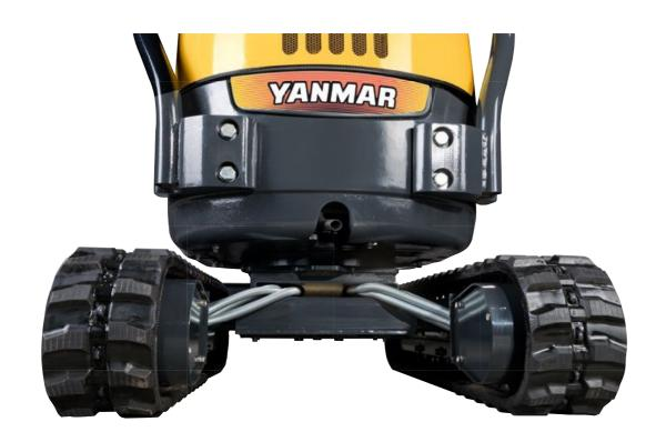
The ViO12 has an operating weight of 1220 kg and the longest undercarriage of its class with 1440 mm. This results in a real improvement of the operator's comfort. He benefits from a smoother drive and increases his productivity.
