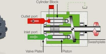
Unlike industry standards for this category of machines, Yanmar is using variable axial piston pump which adapt the flow and the pressure to the load, allowing smoother operation and improving the comfort of the operator. The pump flow of 2 x 11 l/mn and its high working pressure (210 bar) also enable to improve the productivity of the machine and its speed in working motion.
