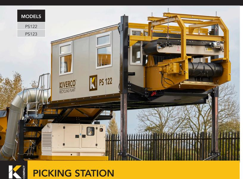
The Compact PS Picking Station range combines air separation, magnetic separation and manual sorting – all in one compact unit:
